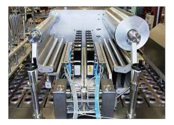
The MULTILINE is as standard equipped with a volumetric dosing device for accurate dosing of liquid and semi-liquid products. Adjustment of the filling volume takes place from the touch screen panel.
